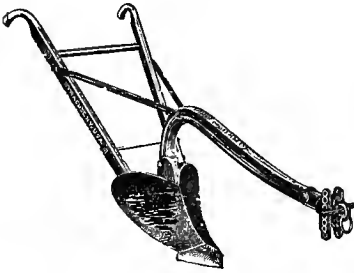
FIG. 75. Middle breaker plow. Sometimes used in constructing irrigation and drainage ditches.
